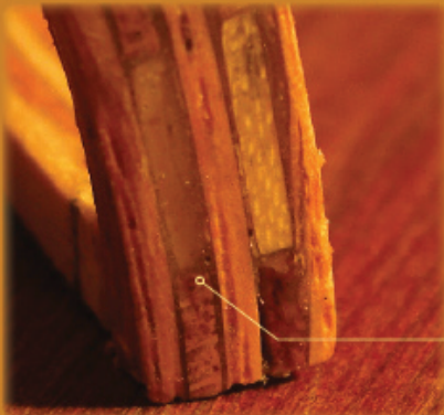
Overlapping Glue Laminated Strips Create Strong Connections and Corners
